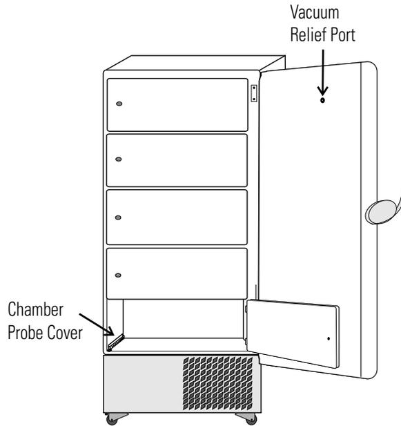
**Figure 1-4.** Vacuum Relief and Probe Cover Location
